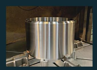
EthosEnergy currently holds the largest inventory in the USA of OEM-recommended 18Mn18Cr retaining rings for generator rotors, including eight different sizes.
