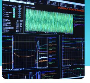
Automated combustion tuning for two GE Frame 9FA gas turbines minimizes unplanned outages
